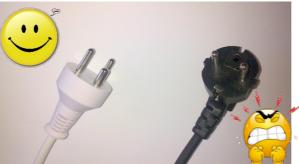
• Mains cables with 2-pin plugs are not earthed and must NOT be used (see picture). Throw them away. The correct plugs can be obtained through the electronic workshop (Incuba)
